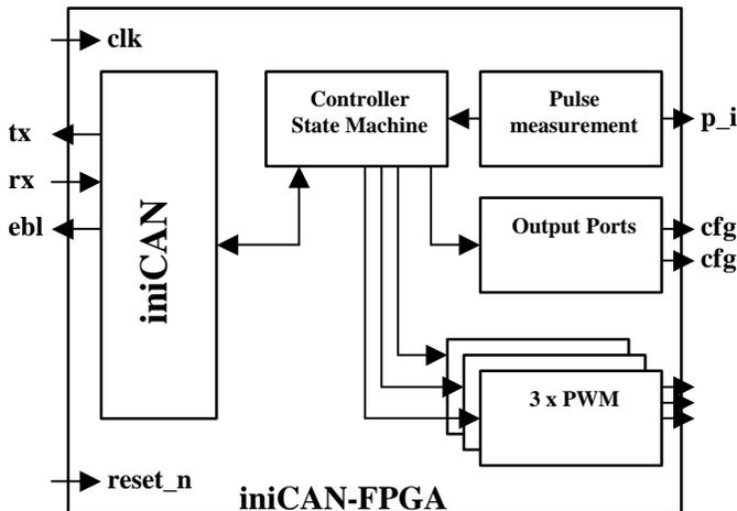
While the iniCAN is handling the CAN protocol, the 'Controller State Machine' decodes the incoming CAN messages and routes the data to the 'Output Ports' or one of the 'PWMs'. Moreover, when a pulse has been detected by the 'Pulse Measurement' unit, a message is generated and sent over the CAN bus.
